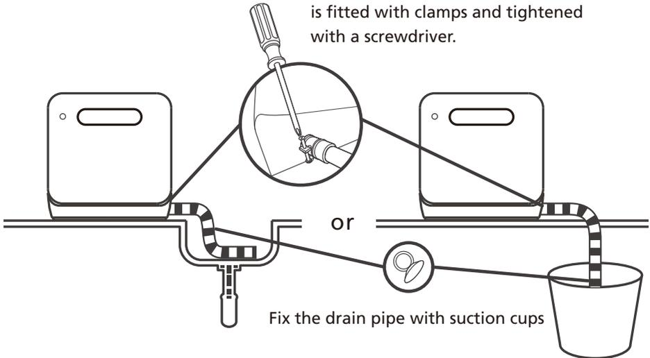
The connection of the drain pipe: Put end of the drain into a sink or bucket.
