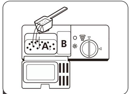
**2** Add detergent into the larger cavity (A) for the main wash cycle .
