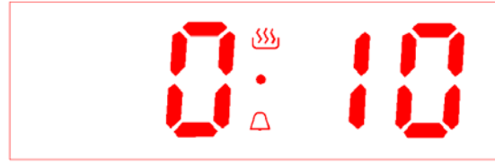
Pic 12 Alarm clock time over diagram (alarm clock icon flickering)
