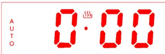
Pic 14 Cooking time setting initial state
