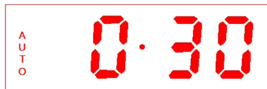
Pic 17 Cooking time over diagram (All the icons flickering)
